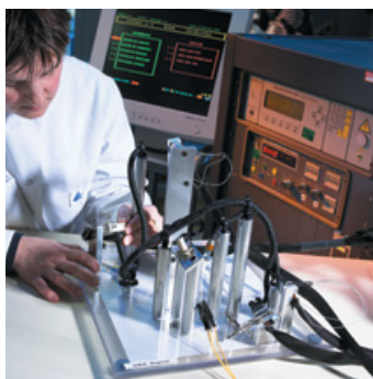
▲ AUTOMATIC CONTINUITY & INSULATION RESISTANCE TEST
